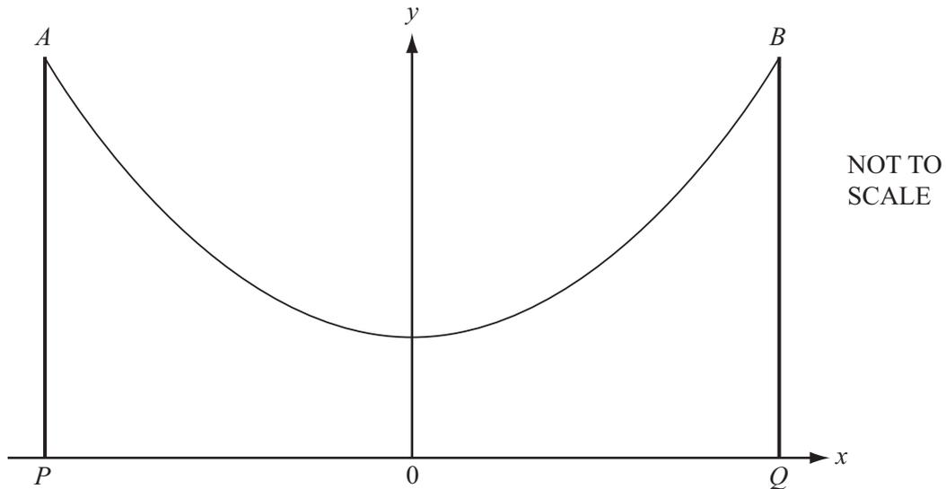
The diagram shows two vertical poles ( $AP$  and  $BQ$ ) that support the ends ( $A$  and  $B$ ) of a hanging chain. The chain is symmetrical about the  $y$ -axis. The poles are each 7.52 metres high and are 4 metres apart. The lowest point of the chain is 2 metres above the horizontal ground ( $PQ$ ). The units are in metres.
